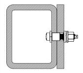
6. Remove the tightening tool and the installation of the Hobson ONESIDE™ bolt is now complete.
