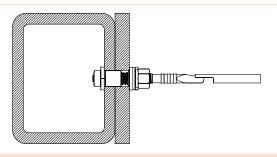
**4.** Slide in the components on the bolt and snug-tighten the nut.
