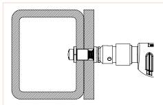
**5.** Remove the installation tool from the joint and use a torque wrench or other means to tighten the nut to the desired tension.
