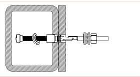
**3.** Rotate the installation tool 180° to unfold the washer. Pull the installation tool back to press the washer against the back of the joint.
